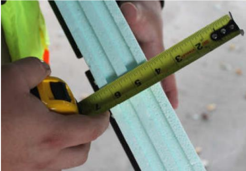
Thickness of insulation - 2\frac{3}{8} "
